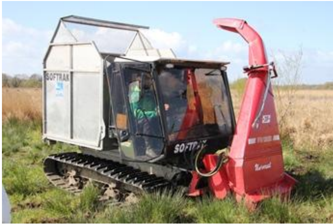
Figure 5.9. The Loglogic Softrak harvesting machine (Photo: Ü. Kask)
