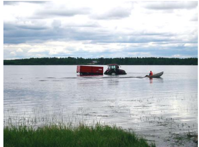
Figure 5.10. Specially equipped Valtra C150 with a trailer in tow can mow reed in the lake ( http://www.valtra.com/news/405.asp )
