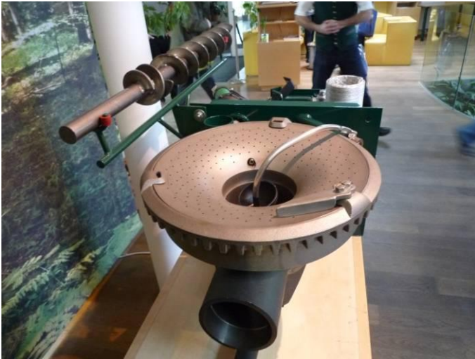
Figure 4.10. The ring nozzle burner (Photo: Ü. Kask)
