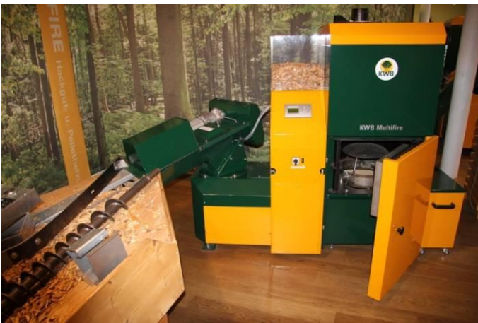
Figure 4.11. KWB Multifire boiler, Austria (Photo: Ü. Kask)
