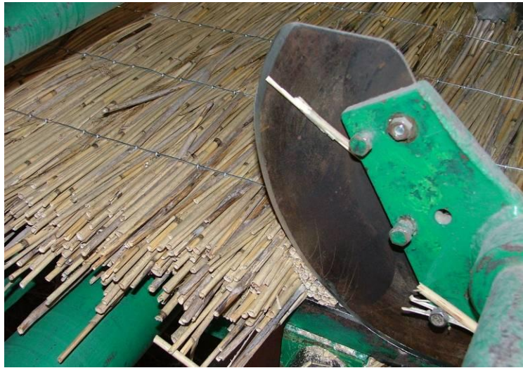
Figure 3.10. a Cutting of the ends of the reed board
