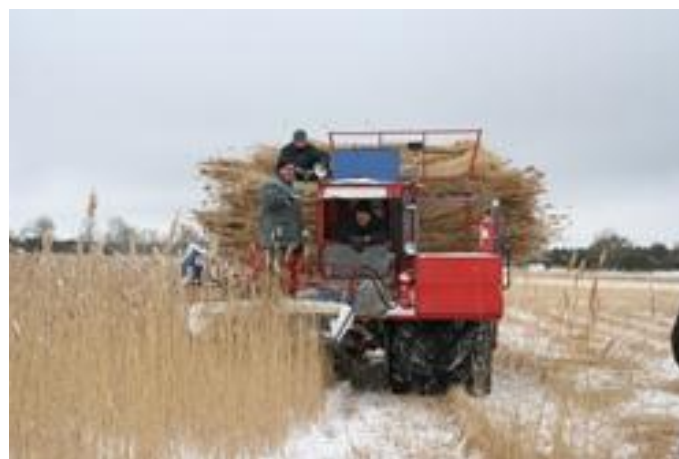
Figure 5.8. Reed cutter Seiga BCS (Photo: Ü. Kask)
