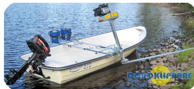
Figure 5.4. Reed mower mounted on a small boat Doroklippenpen Hymo ( http://doroteamekaniska.se/hymo2.html )
