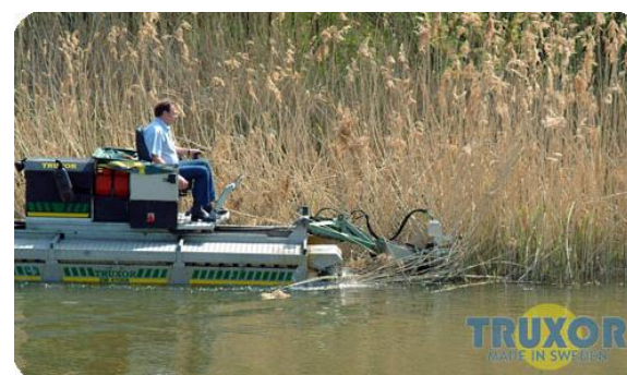
Figure 5.5. Floating mower Truxor Doroklippen ESM 2100 ( http://doroteamekaniska.se/2esm2100.html )
