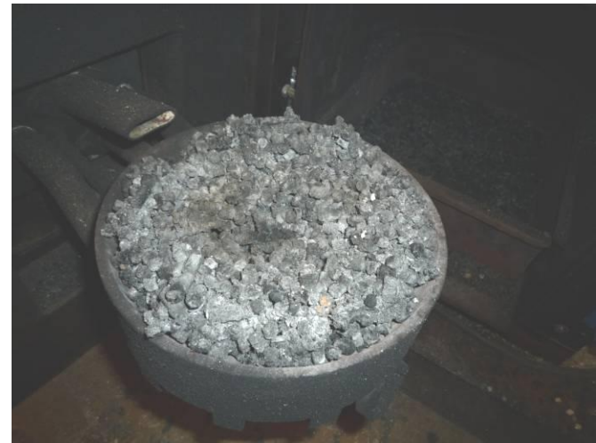
Figure 4.14. Combustion residues after test (Photo: Ü. Kask)
