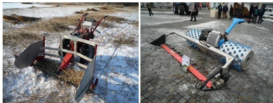
Figure 5.3. Small engine-driven BCS mower (left), mower with a wide header (right)
