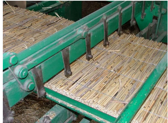
Figure 3.10. b Sewing of the reed board
