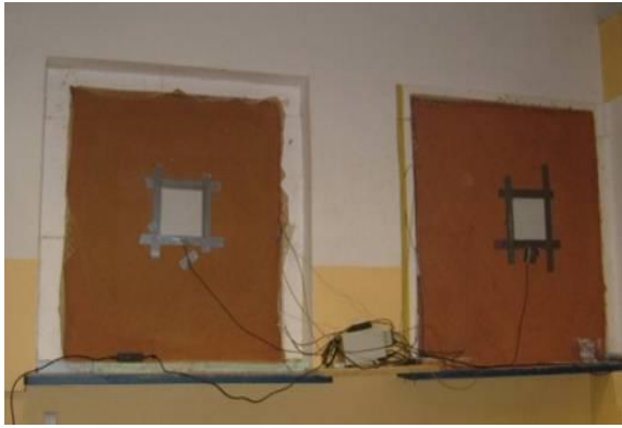
Figure 3.14. Heat flow plates to measure the heat transmittance and thermocouples to measure the air-temperature inside and outside
