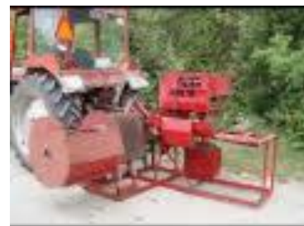
Figure 3.7. A machine for cleaning reeds, powered by a tractor engine
