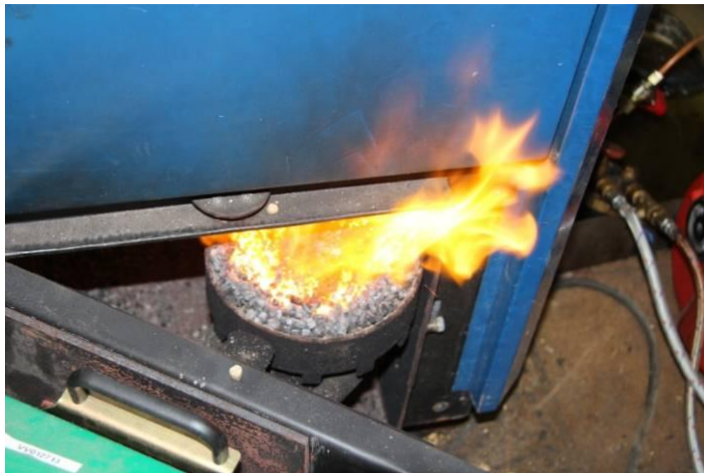
Figure 4.13. Pellet burner BioLine 25 (Sweden) (Photo: Ü. Kask)
